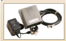
The PA-16 is another ultra low noise, mast mounted pre-amp system that provides a gain of 16 db and a 2.5 dB maximum noise figure.
