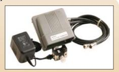
The PA-18 is an ultra low noise, mast mounted pre-amp system that provides a gain of 15 db and a 2.8 dB maximum noise figure.
