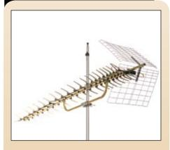
This high performance UHF antenna has a higher gain and a smaller beam angle than conventional Yagi antennas. The reflector grids create an improved front to back ratio with shorter construction while the 91 elements truly make it one of the highest gain UHF antennas available.
