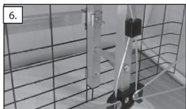
5. Note: adjustable U bolt mast clamps face the rear
