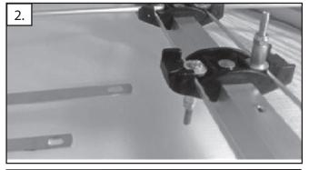
2. Attach combiningbars to the bindingposts on the antenna (bow tie) elements. Tighten using supplied wing nuts. This electrically joins both halves of the antenna.
