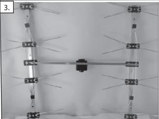
3. Left, both sets of elements joined with the combiner bars. The transformer is in the center.
