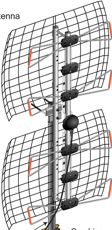
1. Install the two antennas on a single mast, with at least 18 inches (2-4 ft. is recommended) between each antenna.
