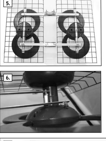
**5.** Both halves of antenna joined with cross braces attached to the rear of the reflectors. Note: adjustable U bolt mast clamps face the rear
