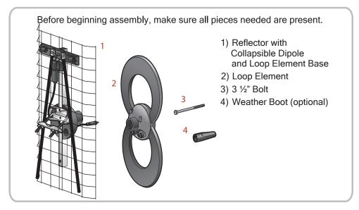
Required, not included: Coaxial Cable, Medium-sized Cross Point Screwdriver.
