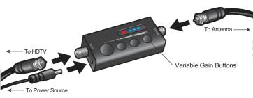
Over amplification may reduce picture quality. Install the antenna without the amplifier first.
