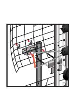
Attach zip tie and connect coax cable to TV or converter box:
