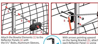
on the Swing Bracket (5), attach to each Reflector Panel (1) using the Swing Bracket Hardware (5). ighten the hardware.
