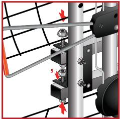
With all coaxial cable connections pointing downward on the Combiner (7) attach one panel at a time to the Crossbar (4) using the Flange Nuts (5). Adjust the Reflector Panels (2) so they are parallel to the CrossBar (4). Tighten the hardware (5).
