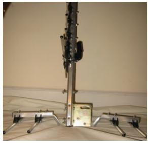
Attach brass colored tilt bracket assembly using supplied bolts and wing nuts to antenna boom as shown.
