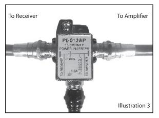
Important: The power inserter sends power UP your down-lead to drive the amplifier mounted on or near your antenna. The power inserter can be located anywhere in your house, but is usually near your TV. The down-lead also brings the digital antenna signal into your house and the signal passes through the inserter to your TV/Digital Receiver. This eliminates any need for a 110VAC wall power source close to your antenna.
