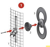
Thread coaxial cable through reflector (1) and hole in base (2) and connect cable to connector on back of loop element (3). Secure reflector, base and loop together with 3 1/2" bolt.
