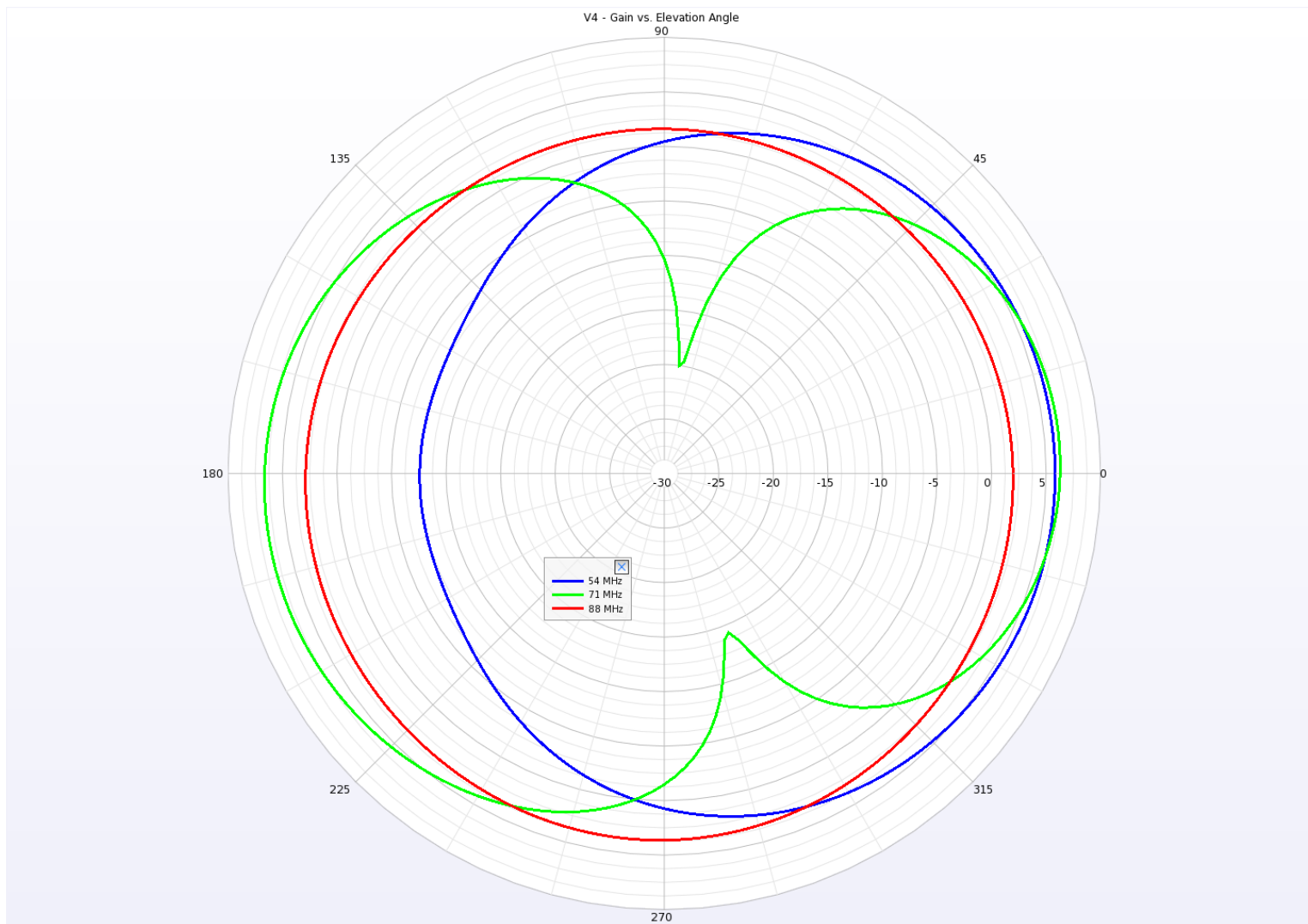
Illustration 2: V4 - Gain vs Elevation Angle.
