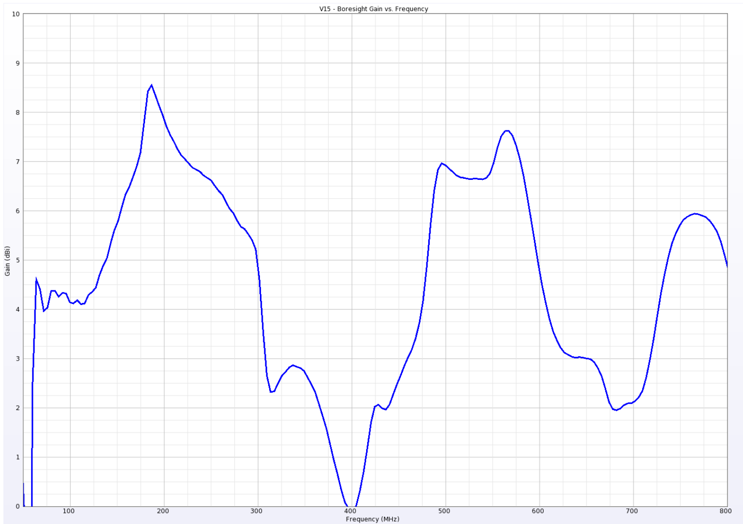
Illustration 7: V15 - Boresight Gain vs. Frequency. Note that peak gain is not on boresight at some UHF channels. Refer to polar plots.
