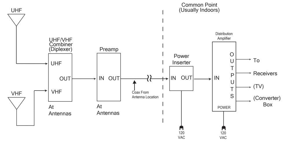
Combining Separate Band Antennas - Using a Preamp Plus Distribution amp
