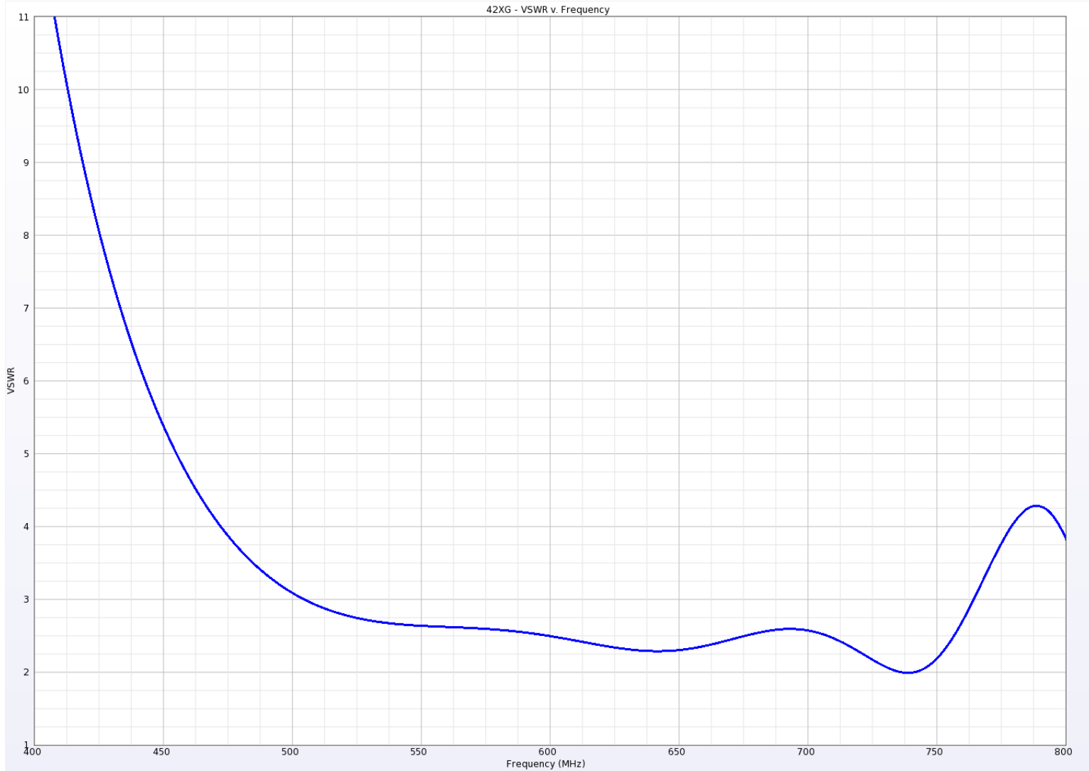
Illustration 4: 42XG - Computed VSWR vs. Frequency. No balun. 300 ohm line reference.
