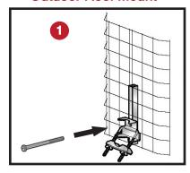
1. Feed the 45%" threaded bolt (2) through the mast clamp assembly (5).
