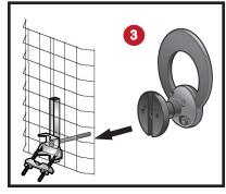
3. Attach the assembled antenna onto the reflector (1) by inserting the threaded bolt (2) into the loop element base (3). Tighten bolt. Attach coax cable to loop element.
