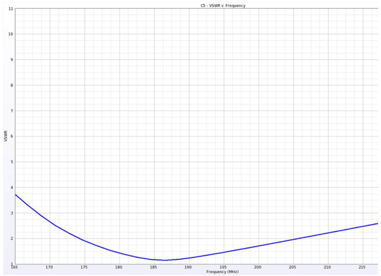
Illustration 5: C5 – Computed VSWR versus Frequency. Balun neglected. Assume 300 ohm line impedance.
