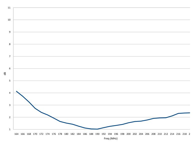
Illustration 6: C5 - VSWR versus Frequency measured using HP/Agilent 8510C VNA with antenna 10 ft above dry concrete.
