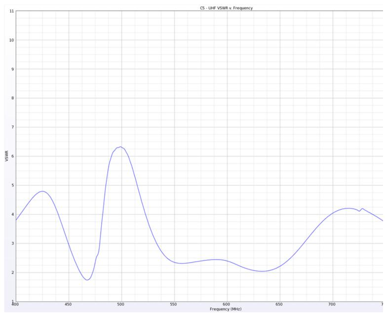
Illustration 7: C5 - Computed UHF VSWR versus Frequency. This is out of band response for this antenna.
