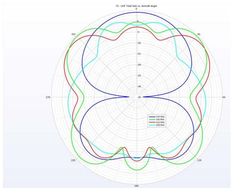
Illustration 8: C5 - UHF gain versus azimuth. Out of band response.
