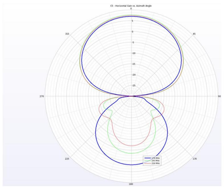
Illustration 3: C5 High VHF Horizontal Gain versus Azimuth Angle. Note: Side lobes lower than total gain of previous
