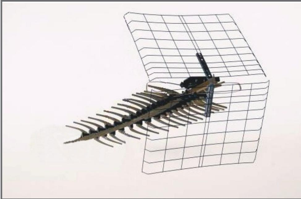
This uni-directional, Yagi style antenna is intended for long range applications ranging from 15 - 60 miles from the transmitters. Its 43 elements create a powerful 15.7 dBi gain with a front to back ratio of 27dB.
