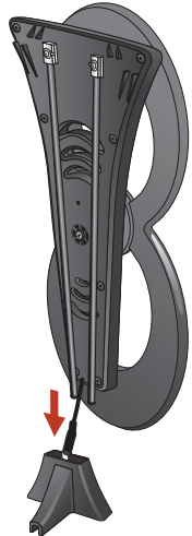
Connect Coaxial Cable (sold separately). Pull Weather Boot over connection.
